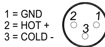
Fig2. XLR Bal Input / Output Pin-out
